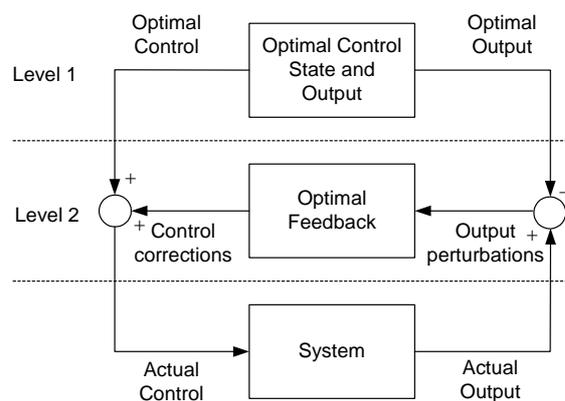
Fig. 1. Optimal control incorporating optimal feedback design
